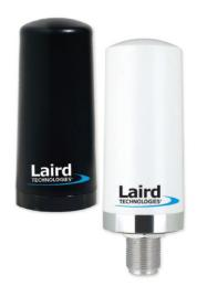
Laird Technologies' unique Phantom® antenna operates simultaneously in the 698-960 MHz and 1700-2700 MHz bands, making it ideal for 4G/3G applications. The mechanically robust design is suitable for both indoor and outdoor applications with wide bandwidth and a low angle radiation pattern that is superior to traditional gain antennas in most applications. The antenna is ideal for both ceiling and surface mount applications.
